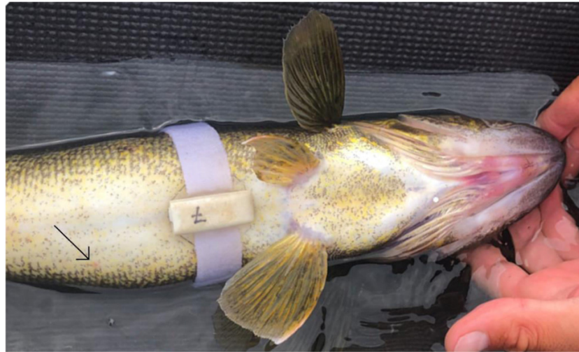
Fig. 1. Walleye ( Sander vitreus ) with the Axy-Depth tri-axial accelerometer positioned ventrally between the pelvic fins and attached around its body. The Velcro strap had a quick release clip positioned dorsally (not pictured), which would release the strap with a sharp tug from the attached line. The arrow points toward the approximate venting location.
